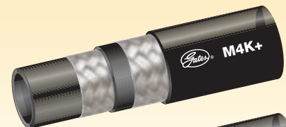
Example of 2-Wire Braid Construction.
