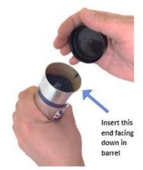
4. Insert the open end of the grease cartridge first
