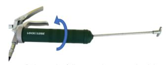
7. Release the follower rod to retract back into the barrel by pulling the rod out of the locked position
