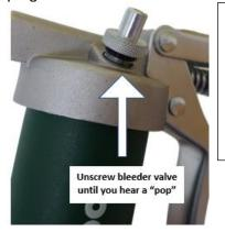
(If your grease gun has a push button bleeder valve, push down while pumping.
